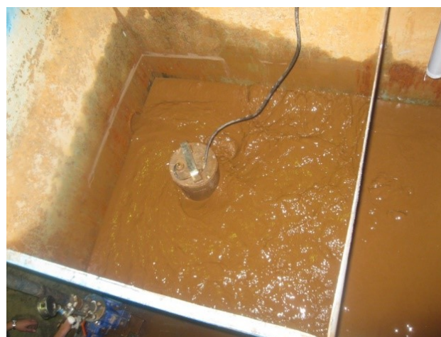
Figure 7: Large slurry tank with blender pumps
