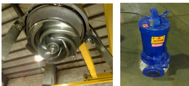
Figure 6: The semi-open impeller and pump used to mix the ingredients in the tank
